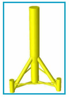
Figure 2.11 Illustration of a Tripod Foundation
