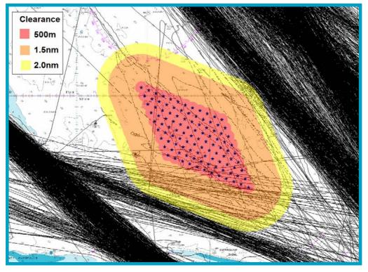
Figure 14.14 Assessment of Impact on Radar
