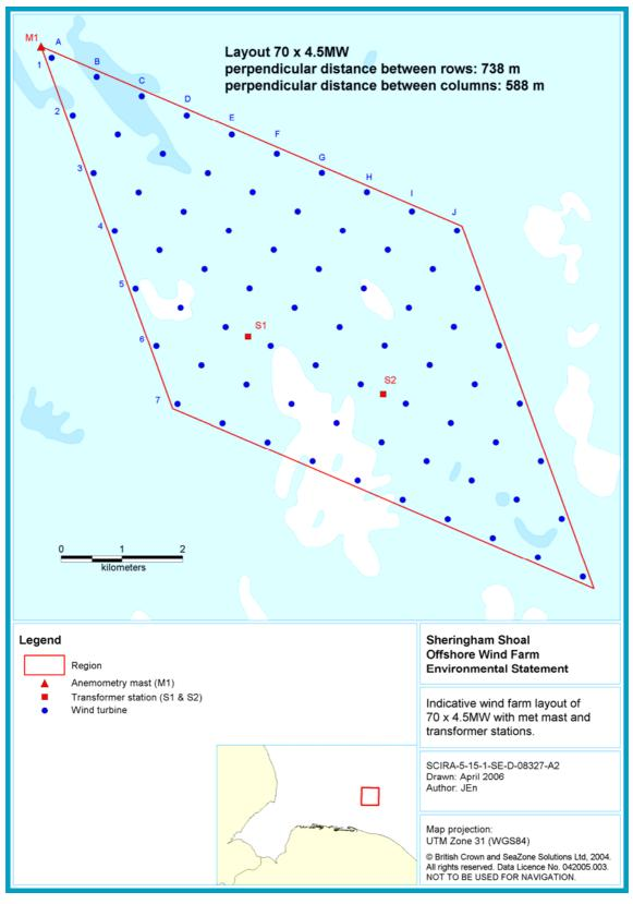
Figure 2.5 Indicative 70 x 4.5 MW Wind Farm Layout, met mast and transformer stations
