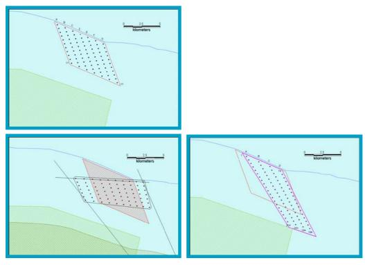
Figure 16.1 Original lay-out, stretched lay-out and radial lay-out, as assessed by QinetiQ in term of impact on clutter and shadowing. The original lay-out proves to be best.
