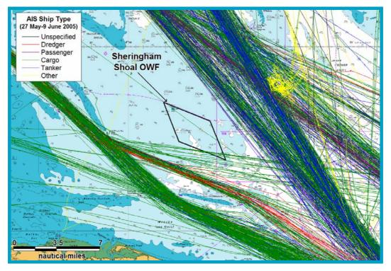
Figure 14.5 Tracks from Additional 14-Day AIS Survey
