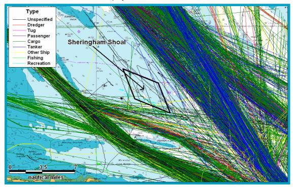
Figure 14.2 Overview of Tracks recorded during Survey (28 Days)
