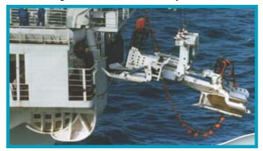
Plate 2.27 Cable plough behind tow vessel
