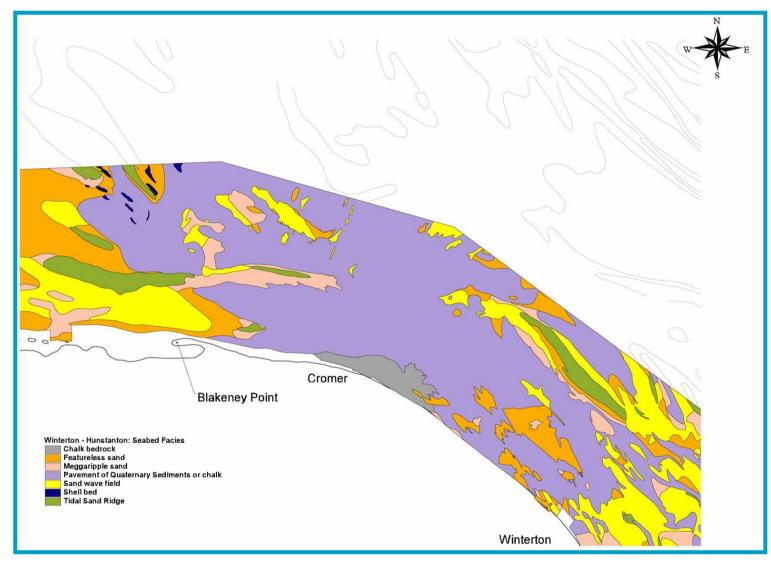
*Figure 6.5 British Geological Survey seabed facies Source: HR Wallingford (2002)*
