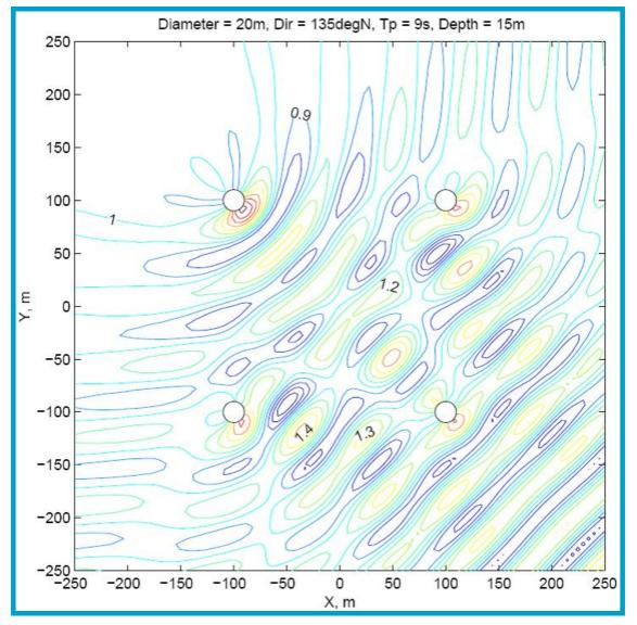
*Figure 6.20:* Wave scattering from 20m diameter cylinders at 200m spacing Souce: derived from Ohl et al (2001)
