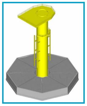
Figure 2.13 Illustrative gravity base foundation
