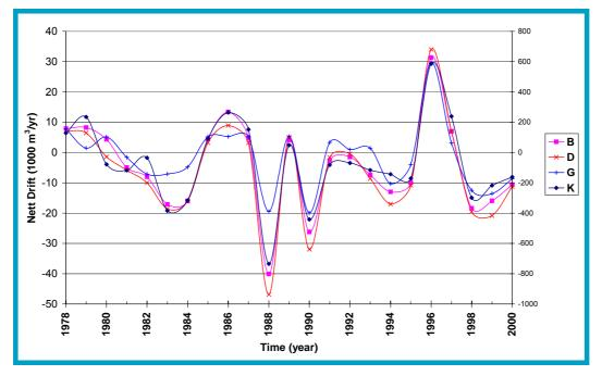
*Figure 6.18: Estimated annual net potential longshore drift rates for four points along the North Norfolk coast;* 1978 to 2001 Source: HR Wallingford (2004)
