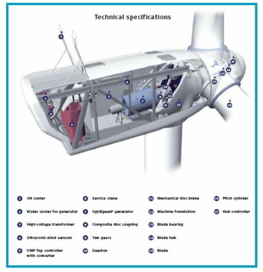
Figure 2.2 A Typical Nacelle Layout (Courtesy of Vestas Wind Systems A/S 3MW))
