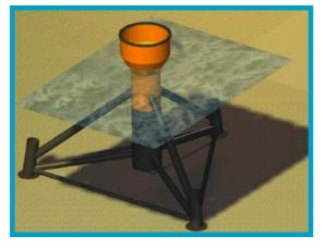
Plate 2.13a, b and c Illustrative multi pile foundations
