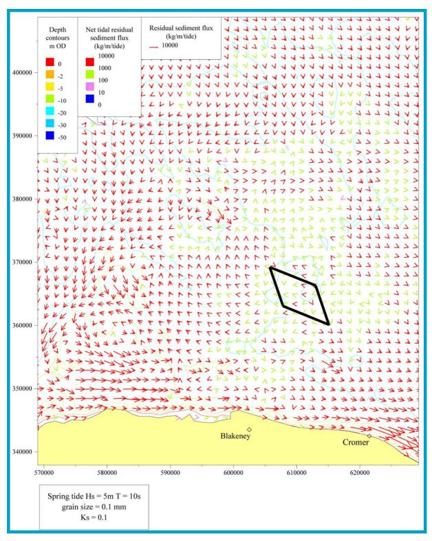
*Figure 6.14:* Nett sediment flux patterns; spring tide with 5m/10s storm waves (0.1mm sand) Source: HR Wallingford et al (2002)
