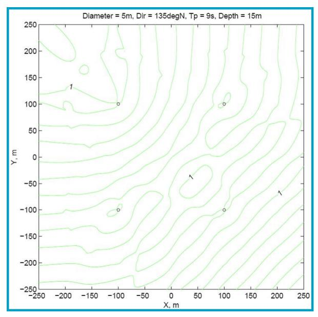
*Figure 6.19: Wave scattering from 5m diameter cylinders at 200m spacing Source: derived from Ohl et al (2001)*
