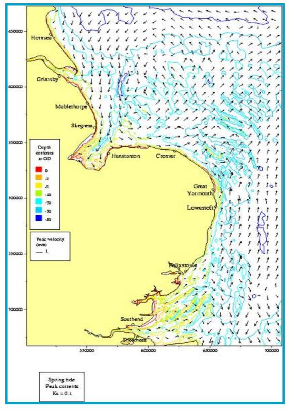
Figure 6.3 Peak spring tide currents, Southern North Sea Source: HR Wallingford et al (2002)
