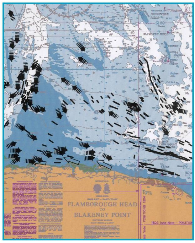
*Figure 6.16: Combined seabed sediment transport indicator map Source: HR Wallingford et al (2002)*
