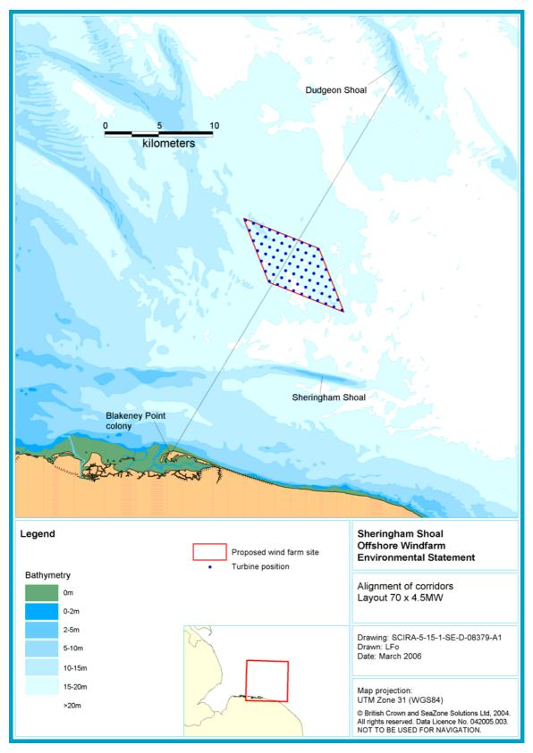
*Figure 8.18* Corridors between the wind turbines are aligned with the prevailing NE-SW flight direction of terns through the proposed wind farm site. The layout shown is 70 x 4.5 MW.
