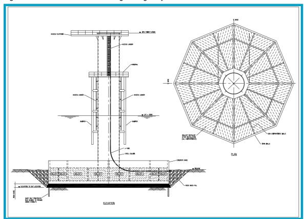
Figure 2.14 shows an indicative design of a gravity base foundation.
