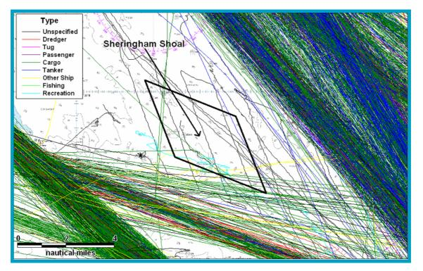
Figure 14.3 Detailed View of Tracks relative to Sheringham Shoal Offshore Wind Farm Site
