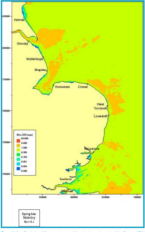
*Figure 6.10* Seabed mobility – maximum mobile grain size under spring tides Source: HR Wallingford et al (2002)
