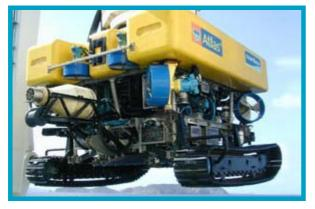
Plate 2.25 Jet equipped remotely operated vehicle
