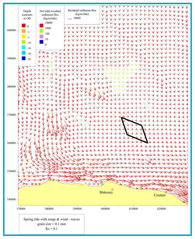
*Figure 6.15:* Nett sediment flux patterns; spring tide with surge (0.4mm sand) Source: HR Wallingford et al (2002)
