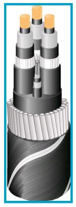
Figure 2.3 Typical 3 Core Copper XLPE Armoured 132 kV Subsea Cable with fibre optic cable (Courtesy of ABB)
