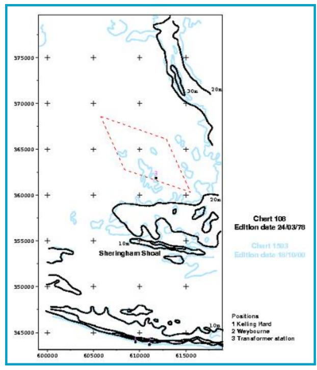
*Figure 6.8 Comparison of landfall seabed contours*
