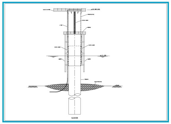
Figure 2.10 shows an indicative design of a monopile foundation.
