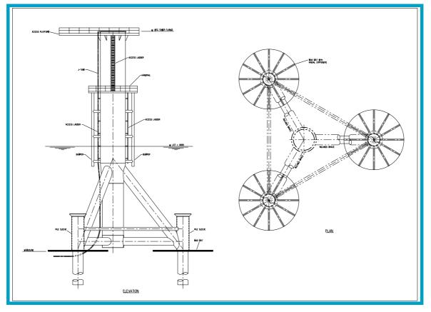
Figure 2.12 Indicative design of a tripod foundation
