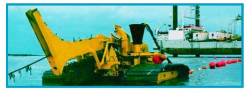
Plate 2.24 Self propelled plough
