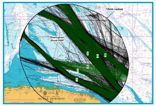
Figure 14.7 90% Lanes overlaid on Survey Tracks
