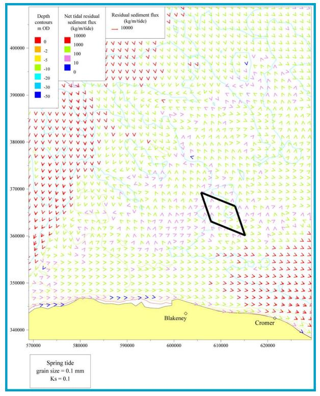
Figure 6.13 Nett sediment flux patterns; spring tide (0.1mm sand) Source: HR Wallingford et al (2002)
