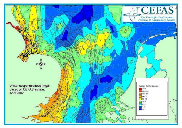
Figure 6.12 Mean winter suspended sediment concentrations (units: mg/l) Source: HR Wallingford et al, (2002)
