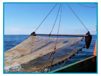
Plate 10.1 The 7m steel beam trawl used in the July 2005 and the September 2005 fish survey.
